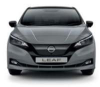
A: Overall length: 4 490mm | B: Wheelbase: 2 700mm | C: Overall width: 1 788mm | D: Overall height: 1 540mm
